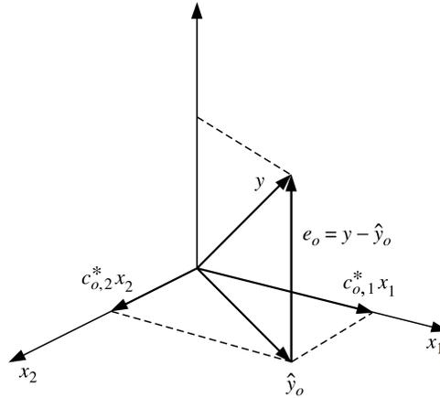
Figure: Illustration of the orthogonality principle.  $x_m \perp e_0, m = 1, 2$ .
