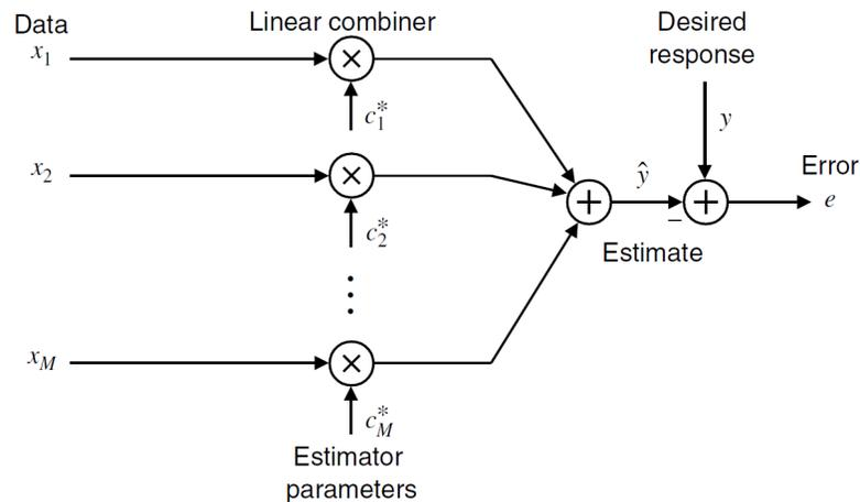
Figure: Block diagram of the linear estimator.
