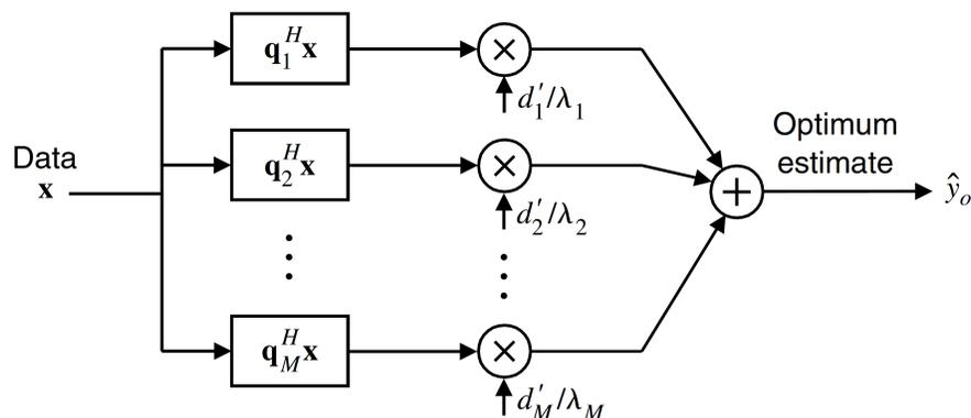
Figure: Principle-components representation of the Optimal linear estimator.
